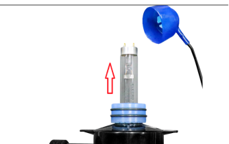
Gently slide the lamp out ensuring that no pressure is applied to the quartz sleeve
